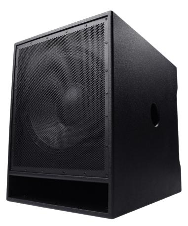
**Integrated, comprehensive DSP is included.** Processing includes high-pass and low-pass filters as well as multiple protection systems and limiters to control all manners of driver overload, including thermal, excursion and clipping. The protection systems effectively prevent overheating of the voice coils and minimize long-term thermal compression while having virtually no effect on the transient response and peak output of the loudspeaker.
